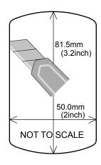
3. Insert EDGE EQ into hole of guitar. (Two clamps must be fully unfastened)
