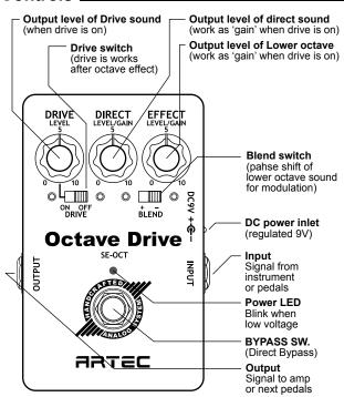
Battery: 9V Alkaline 6LR6l or 6F22DC power supply: 9V regulatedPower consumption: 5mA
